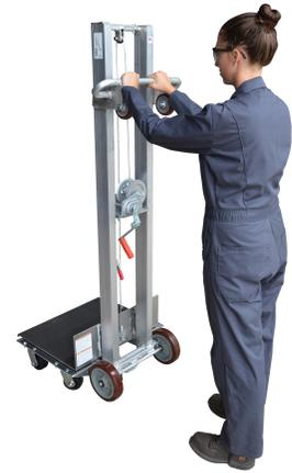
Lightweight unit ideal for delivery trucks and vans. Hand winch operation with automatic positive lock for raising and lowering platform. Ergonomic design allows the operator to load material from ground level without bending over. Smooth maneuvering from one workstation to another. Mold-on-rubber 6" x 2" rear wheels are standard. Capacity is 175 lbs.
