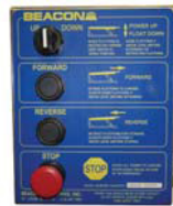
CONTROL STATION BOX
