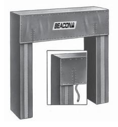
The standard Series 101 dock seal features a fixed 24" head curtain for doors higher than 9 ft. A special design, Series 103, features an adjustable head curtain that can be raised or lowered by a "touch-and-hold" pulley arrangement
