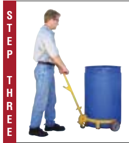
STEP THREE Reattach handle and transport drum to desired location.
