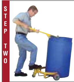
STEP TWO Tip drum up while guiding the base under the drum.
