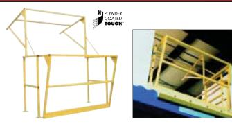
The Mezzanine Safety Gates provide an OSHA required 42" high handrail, 21" mid rail and 4" high kickplate for mezzanines without sacrificing load accessibility. The gate rotates to allow loading and unloading of maximum 48" wide x 48" high pallets. Safety yellow powder coat finish.
