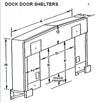
Reinforced Fiberglass Sides and Top: White polyurethane is secured to wood framework.
