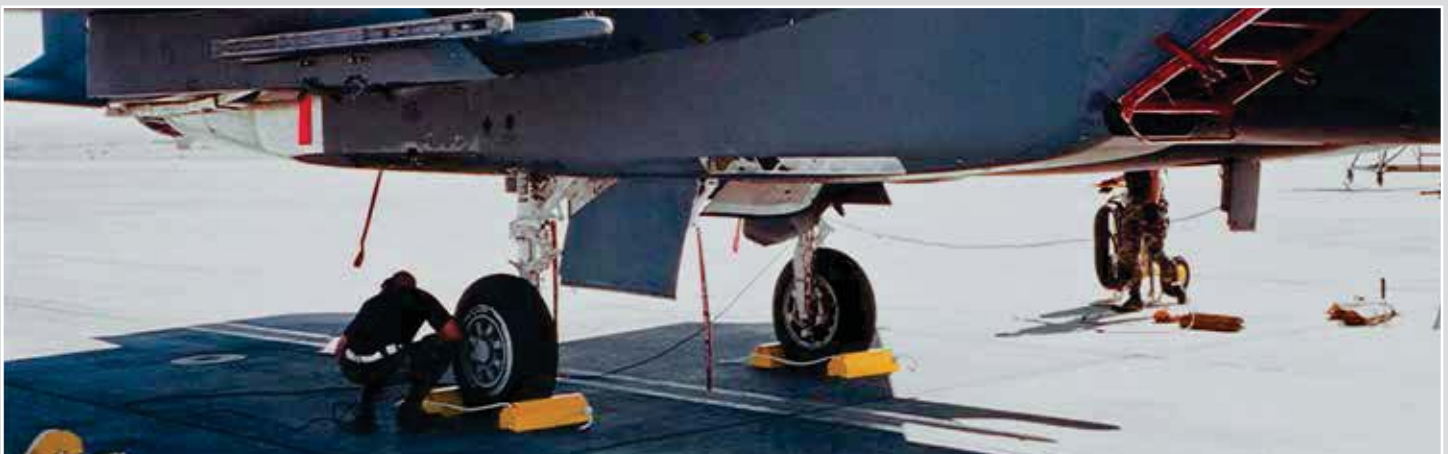
AC6820-LR aviation chocks used on a McDonnell Douglas F-15 Eagle
