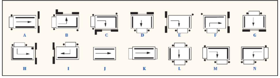
When quoting, Load Transfer Arrangements should be specified to allow the appropriate safety factor for your application.
