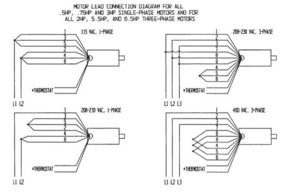
\* The two thermostat leads go to: 1) the grounded side of the transformer secondary, and; 2) the notor relay coll, in either order.
