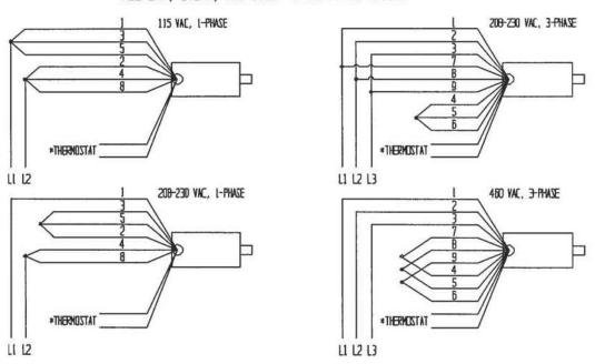
\* The two thermostat leads go to: 1) the grounded side of the transformer secondary, and; 2) the notor relay coll, in either order.
