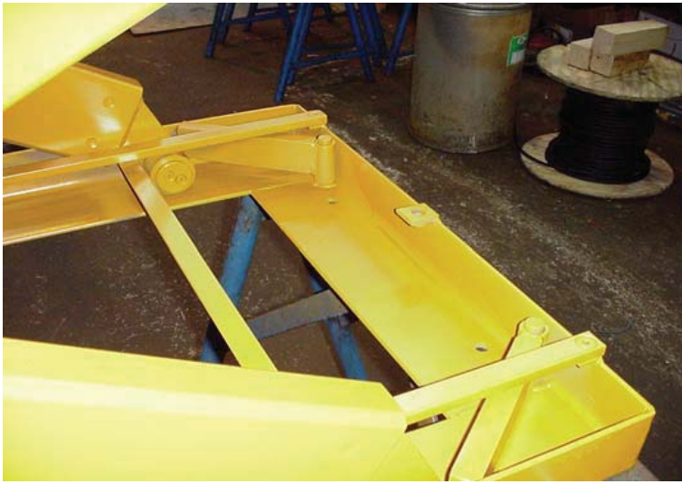
FIGURE 3b - MAINTENANCE BAR OPERATING DETAIL FOR BDSL 90" THRU 144" V.T. & BTSL 72" THRU 144" V.T. ONLY.
