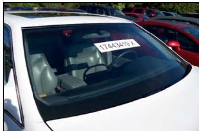
RFID Label Applied to Vehicle Windshield
