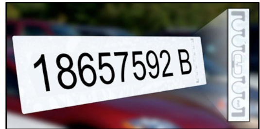
Close Up of RFID Label (Note RFID device in zoomed portion of label.)
