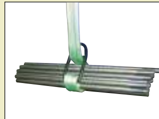
Choker Style Lift (20% Reduction of Capacity)
