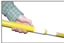
Push Snap Button In and Extend Pole to Desired Length
